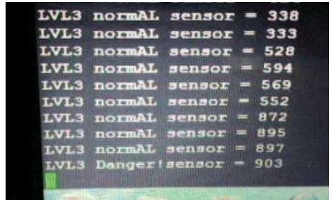
Figure 6: Fire Detection Interface on Monitoring System
